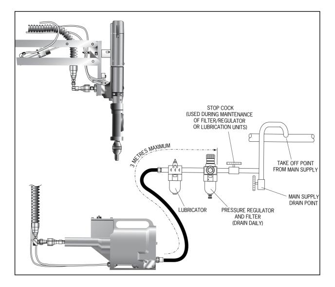
Follow the steps below when connecting the tool to the intensifier and main air supply:
